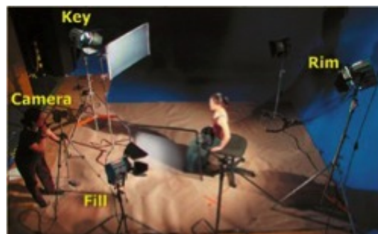
Figure 7.14: The figure shows a setup of the three point lighting illumination process with the three lights. [Birn, 2006, Chapter 5].
