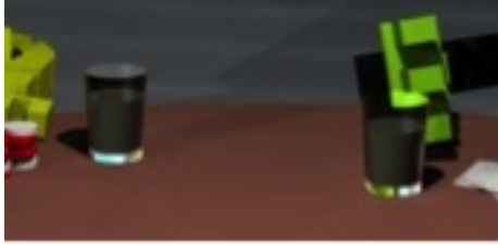
Figure 8.15: Test render with reflection at 2, refraction at 3, max trace depth at 5 and shadows at 2.
